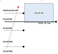
The shaded area represents the temperature range defined by the "heating control differential ON" parameter in case of increasing temperature.
