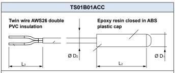
D1 = 9 mm D2 = 4 mm L2 = 49 mm L1 = 1250 mm
